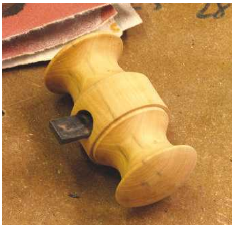
▲ Pic.34 The ebony wedge needs to fit perfectly into the hole in the head so I sand until it is exactly the right width. The wedge is about 15mm long and about 2mm thick at the fat end
